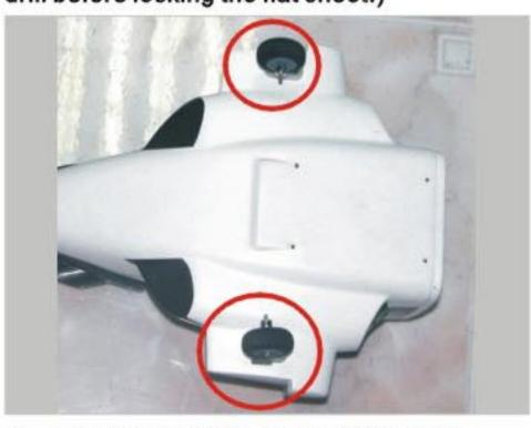
6. 把后起落架左右后轮都锁好 Lock the left/right & rear wheel of back undercarriage tightly.
