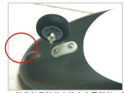
3. 把前起落架装上机壳头罩下部,用自攻螺丝和压片锁住(螺丝: 2\*10, 2 个; 压片: 2\*10mm, 1个)<注意: 钮住压片时要先用手钻钻好1.5的孔位> Insert the undercarriage(front) into the nether of canopy, then lock them by self-threading screws and flat sheet. (Screw: 2\*10, 2pcs; Flat sheet: 2\*10mm, 1pcs) (Remarks: Drill 1.5mm hole by hand drill before locking the flat sheet.)
