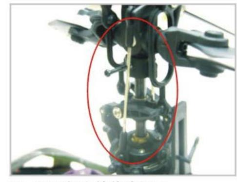
19. 把飞机主转旋头钮下 Rive off the center hub set of helicopter
