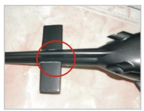
1. 把机壳平尾用AB胶粘上 glue the edge tail of cabin with AB glue.
