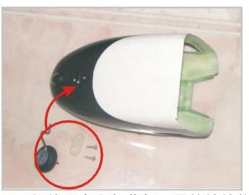
2. 把轮子套上起落架,用轮锁锁住 Hitch the wheel to the undercarriage, then lock them.
