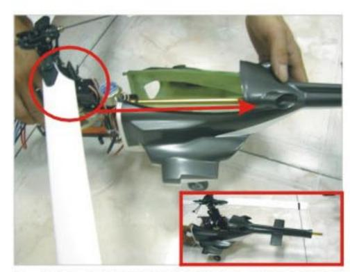
7. 把飞机滑撬和尾箱钮下装进机壳 〈注意:尾拉杆也要取下〉 Insert the landing skid and button of tail box. (Remarks: Please remove the tail push link as well.)
