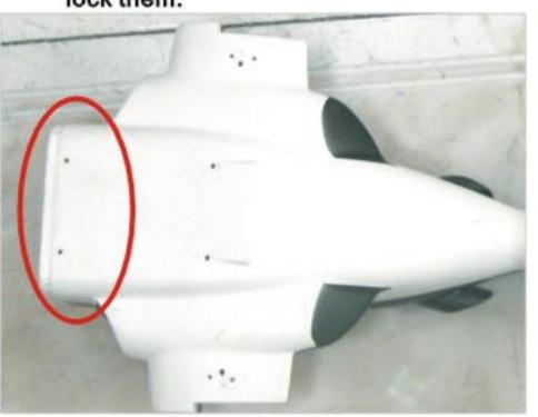
4. 把后起落架装上 Install the back undercarriage.
