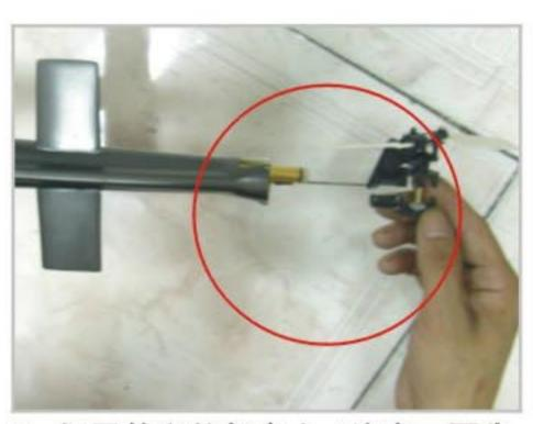
8. 把尾箱和拉杆套上〈注意:要先 把尾摆臂前一个孔剪掉,然后把 拉杆装进尾摆臂第二个孔位〉 Install the tail box and push link. (Remarks: Scissor the front hole of the tail control arm firstly, then insert the push link into the second the hole.)
