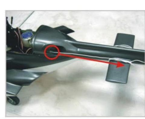
Pull out the receiver antenna from the back hole of cabin, then enlace them on the edge tail.
