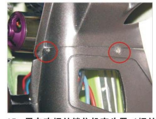
15. 用自攻螺丝锁住机壳头罩 (螺丝: 16. 把机壳尾巴套上 1.4\*5,6个)〈注意:在钮螺丝之前先钻好1mm的孔位,再锁螺丝〉 Lock the cabin by self-threading screws ( Screw: 1.4\*5, 6pcs) (Remarks: Drill 1mm
