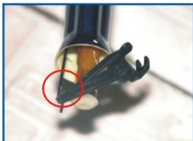
8、把尾摆臂装上尾拉杆 Put the tail suspension arm onto the tail Push-rod.
