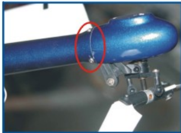
19、用自攻螺丝拧紧(螺丝:1.4*5、3个) Screw it down with tapping screws. (Screw:1.4*5 3PCS)
