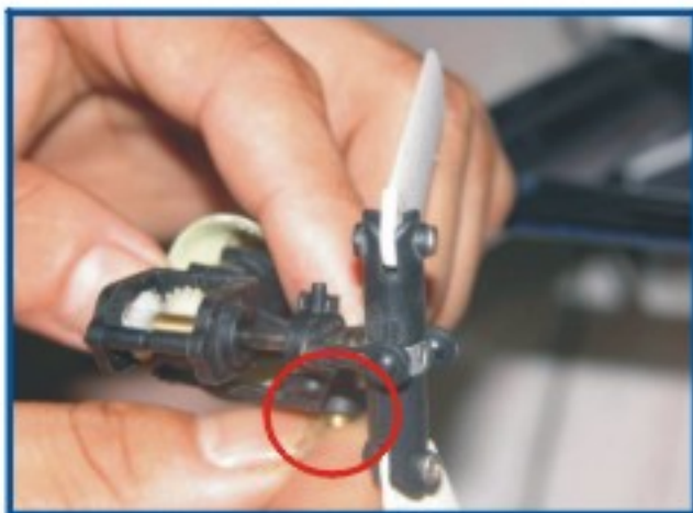
11、把尾摆臂套上 Slip on the tail suspension arm.
