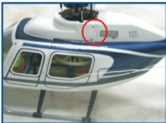
17、用自攻螺丝把机壳头罩拧紧(螺丝:1.4*5、10个) Screw down the canopy with tapping screws. (Screw:1.4*5 5PCS)
