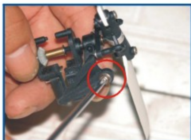
4、用十字螺丝刀把尾摆臂钮下, 也要把尾拉杆取下 Take away the tail suspension arm with the cross screwdriver, and take off the tail push-rod.
