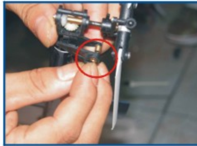
12、用螺丝把尾摆臂固定好 Fix the tail suspension arm with the screws.
