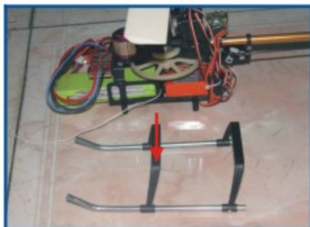
2、用十字螺丝刀把滑撬钮下 Take off the the landing skid with the cross screwdriver.
