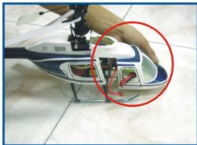
16、在机壳头罩上把座仓用自攻螺丝装好,然后把机壳头罩套上 Put the cabin on the canopy with tapping screws, then cover the canopy.
