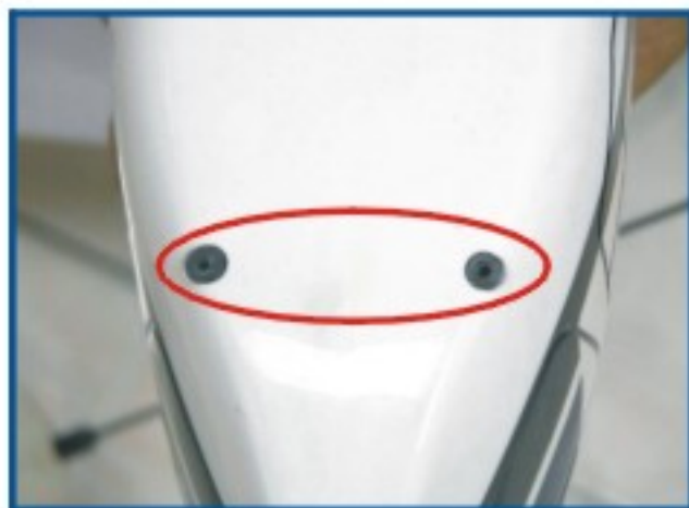
13、把机身对好机壳上四个孔位 Make the body aim at the four hole place of cabin.
