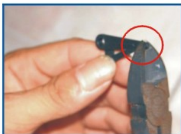
5、用钳子把尾摆臂前一个孔剪掉 Cut off the anterior hole of the tail suspension arm with the plier.
