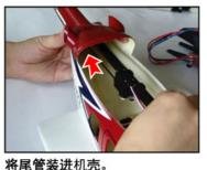
Put the tail boom into the shell.
