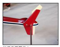
把垂直尾翼装上。 (自攻螺丝: 2\*10mm 2个) Assemble the vertical fin. (Self-tapping screw: 2\*10mm 2PCS)
