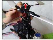
Disassemble the main swivel head with the hex screwdriver.
