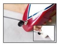
将起落架装在机壳底部。(前后起落架 (自攻螺丝: 2\*10mm 2个) Assemble the front and rear undercar (前后起落架)
