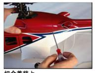
把仓盖装上。 (自攻螺丝1.4\*5mm 4个) Cover the hatch. (Self-tapping screw: 1.4\*5mm 4PCS)
