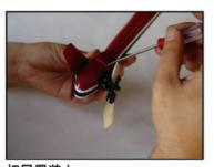
把尾罩装上。 (自攻螺丝1.4\*5mm 3个) Put on the tail cover. (Self-tapping screw: 1.4\*5mm 3PCS)
