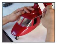
把座仓装上。 (自攻螺丝: 1.4\*5mm 2个) Assemble the cabin. (Self-tapping screw: 1.4\*5mm 2PCS)
