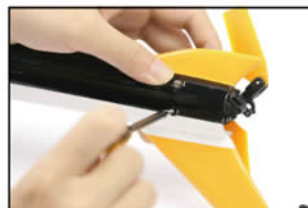
12.将尾齿轮箱组螺丝拧紧 Tighten the screws of the tail gear set
